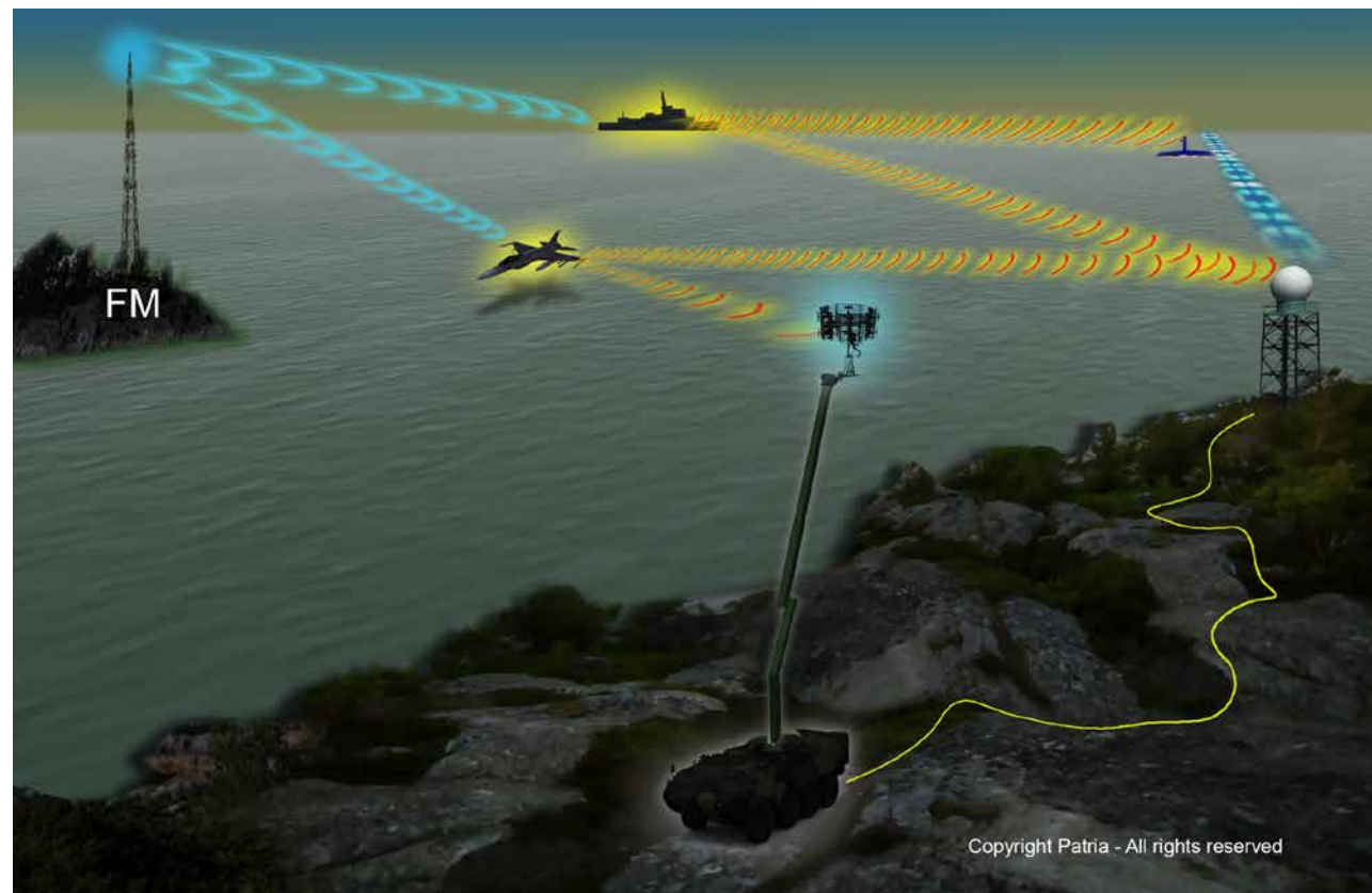
Patria MUSCL. A passive radar system for surveillance, early warning, and critical infrastructure protection by detecting, locating and tracking silently full range of aerial and surface threats in the modern battlefield.
